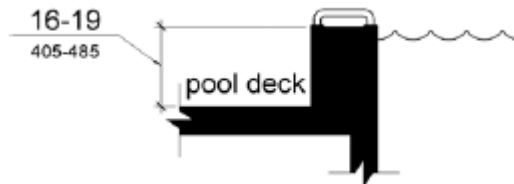
Figure 1009.4.2 Transfer Wall Height
